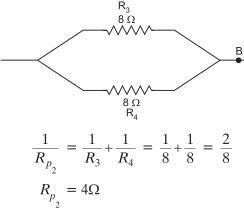
Now  $R_{p_1}$  and  $R_{p_2}$  are in series. So the equivalent resistance between the two points A and B in the circuit is
